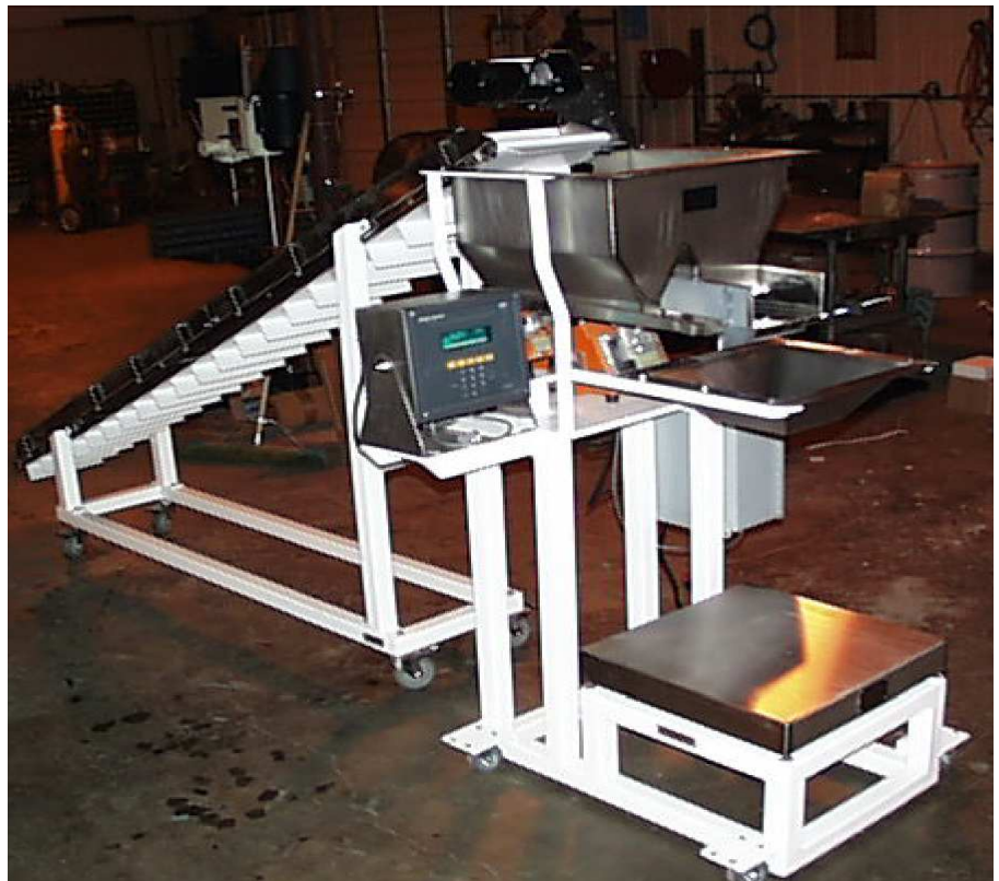
PS-10 Semi-automatic bulk packaging system for a cinnamon sugar topping mix with the portability option
